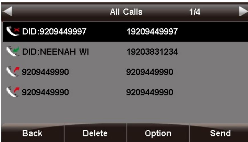
3. You can use the < and > (left and right arrow) buttons to filter by call type: **All Calls**, **Missed Calls**, **Received Calls**, and **Dialed Calls**. The current filter option is shown at the top of the screen.
